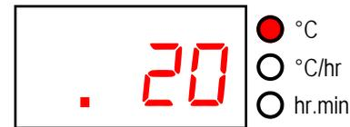
If the left-hand decimal point is on then the keyboard is locked & the ST312 will not respond to the START/STOP key. Press the  $\uparrow$  &  $\downarrow$  keys together & hold down for 5 seconds to unlock.
