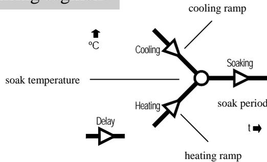
An ST315 firing segment comprises a ramp followed by a soak period. Two segments can be used for simple firing (biscuit firing for example) or up to 9 segments can be used per program for complex firing (crystal glazing or glass-making for example).
