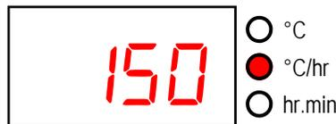
**➡** then displays the ramp rate in the range 1 to 999°C/hr or *FULL* or *End*. This can be altered with the **⬆** & **⬇** keys. The HEATING RAMP or COOLING RAMP lamp on the mimic display will flash.
