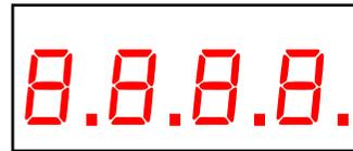
When turned on the ST315 performs a display test by briefly illuminating all of the display digits and all of the front panel lamps.
