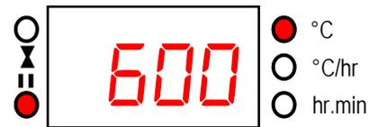
As a warning during pause a double beep is sounded every 10 seconds and the display scrolls PAUSED. The PAUSED lamp to the bottom left of the main display is lit.
