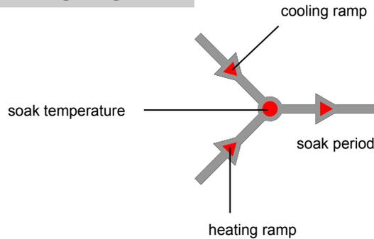
An ST325 firing segment comprises a ramp followed by a soak period. Two segments can be used for simple firing (bisque firing for example) or up to 32 segments can be used per program for complex firing (crystal glazing or glass-making for example).
